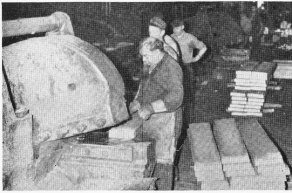
1) When metal is poured into moulds at the Casting Shop, the dirt and impurities float to the top or gate end of the bar. Pete Lesauskas, who can tell an alloy by the sound when it's cut, is shown at the huge Alligator Shears that chop off the gate before the bar goes to the East Rolling Mill. Clarence Andrews and Mike Lawlor help Pete handle the 200 pound bar.
