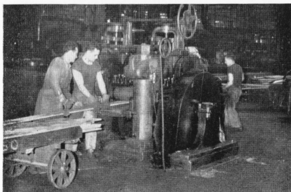
6) Giant cranes gather the bars and take them to the less powerful but faster Running Down Rolls. After successive passes and anneals, the bars are either finish rolled for working into shell cases—or sent to the North Rolling Mill for finer rolling. Lee Rogo and Casimir Szczepanski feed the Running Down Roll while Casimir's son Peter piles the rolled bars on the other side.
