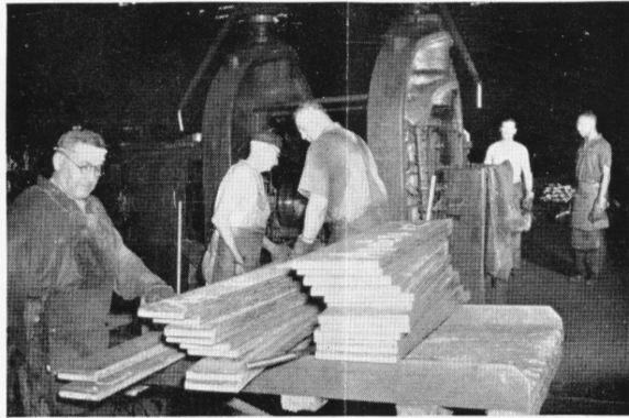
2) Cast metal must be processed by cold working and heat treatment before it can be used. Michael Stere, left, helps Roller George Gentil and George Benoit feed the metal bars between the cylinders of the Breaking Down Rolls that pinch the bars with several million pounds of pressure. Antonio Seabra and Herbert Wolfrey wait to stack the rolled metal as it comes out.
