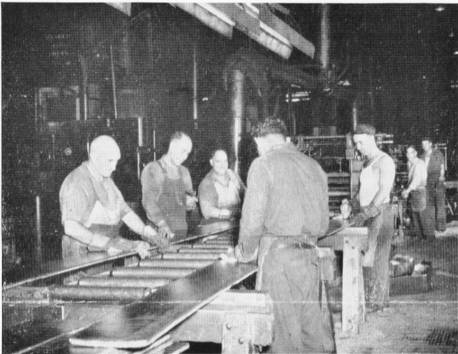
4) Before the annealed bars are rolled again they are cleaned and brightened by the Overhaul Machine in which whirling cutters chip off the surface. Here Louis Scozzajava, Albert Proulx, Joseph Minervini, Daniel Lopes and Antonio D'Azevedo attend the machine. In the background Leonardo DaLapa and Herman Pekrul feed the bars through.
